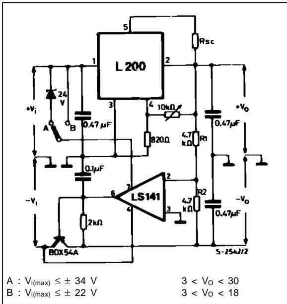
Since the maximum supply voltage of the op amp used is  $\pm 22$  V, when pin 7 is connected to point B output voltages up to about 18 V can be obtained. If on the other hand pin 7 is connected to point A, much higher output voltages, up to about 30 V, be obtained since in this case the input voltage can rise to 34 V.
