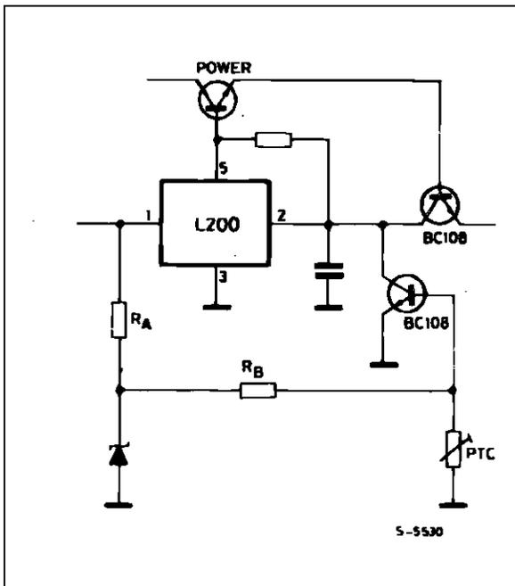
VOLTAGE REGULATOR FROM 0V TO 16V - 4.5A
