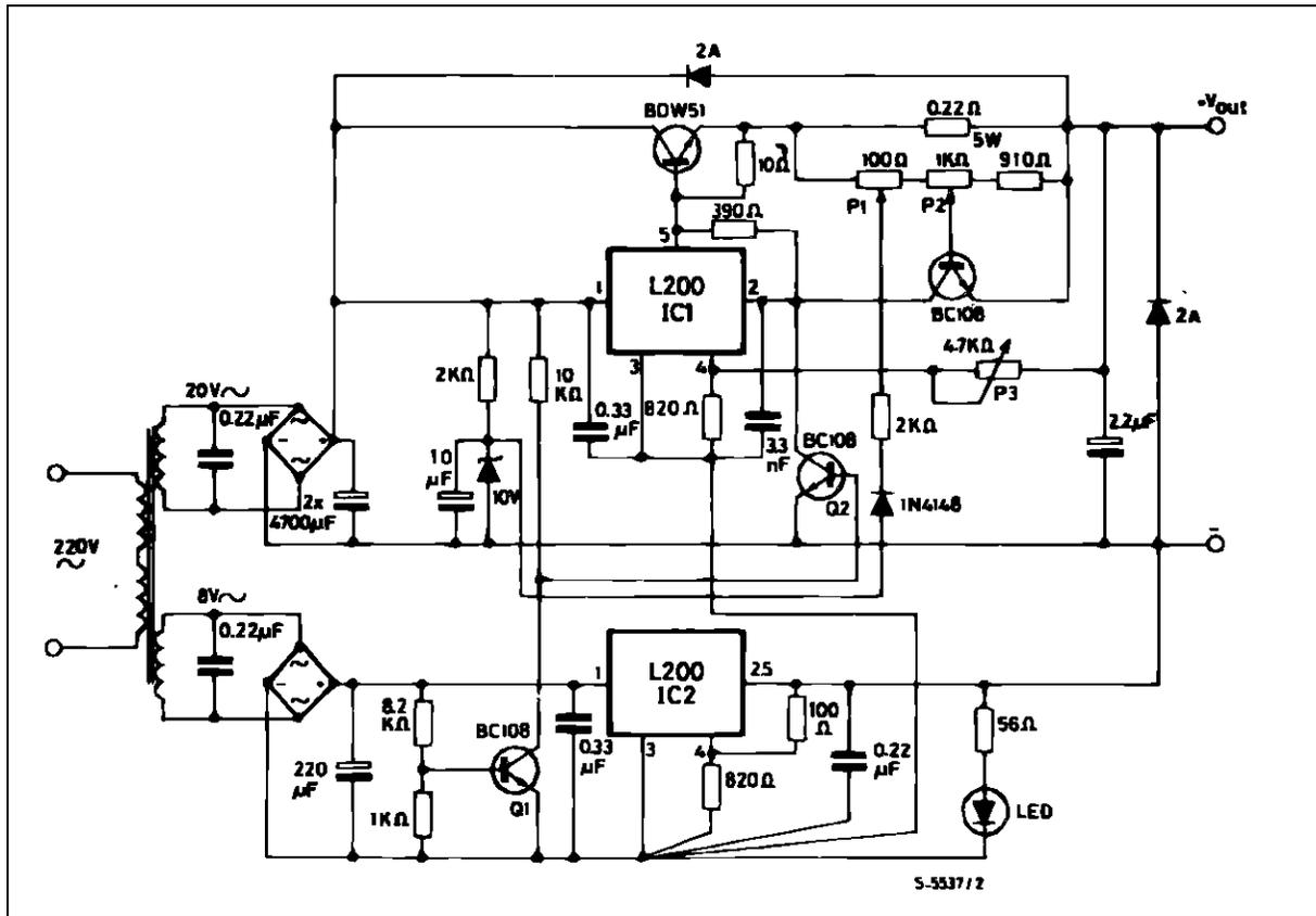
POWER SUPPLY WITH  $V_o = 2.8$  TO  $18$  V,  $I_o = 0$  TO  $2.5$  A
