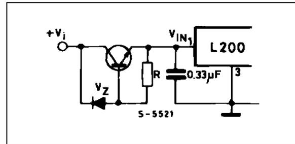
The designer must take into account the dissipated power and the SOA of the preregulation transistor. For example, using the BDX53, the maximum input voltage can reach 56 V (fig. 16). In these conditions we have 20 V of  $V_{CE}$  on the transistor and with a load current of 2 A the operation point remains inside the SOA. The preregulation used in fig. 16 reduces the ripple at the input of the device, making it possible to obtain an output voltage with negligible ripple.
