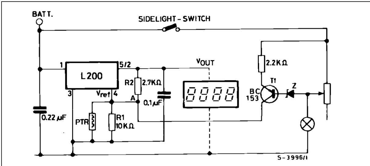
In dusk conditions, when the sidelights are switched on, T1 starts to conduct with its conduction set by the potentiometer wiper at its uppermost position the sidelights are at their brightest and current through T1 would be a minimum. With the wiper at its lowest position obviously the opposite conditions apply.
