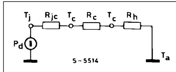
**Note 2 :** In applications where one or more external transistors are used together with the L200, the dissipated power must be calculated for each component. The various junction temperatures can be calculated by solving the following circuit :
